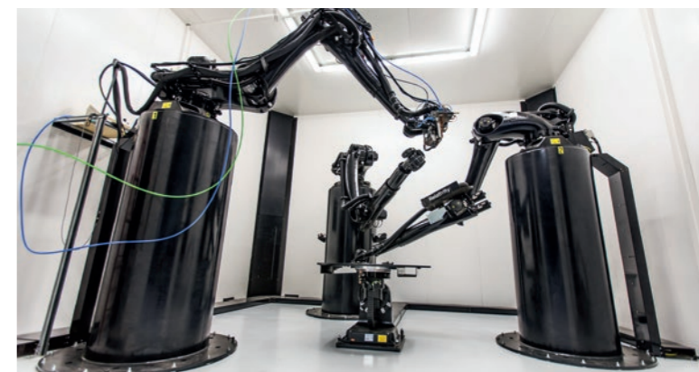
At the heart of Relativity Space's technology is the 3D printer Stargate, which has already produced numerous large-scale rocket components
