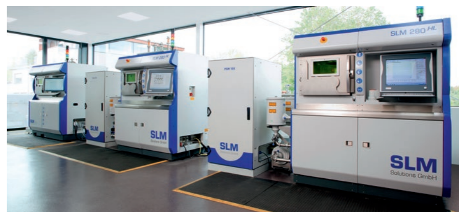
The AM department at Rosswag wants to automate »the small, time-consuming steps«. The machinery includes three SLM 280s from SLM Solutions, an AL3D from Alpha Laser and a small-batch gas atomizer from BluePower, as well as CNC machines and a materials lab.
